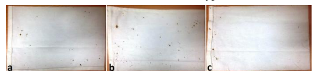
Figure 3 burnt points on cotton in pan 1 in experiments with mulch firebrands at wind speed of a) 6.5m/s, b) 9m/s, c) 14.5m/s.
